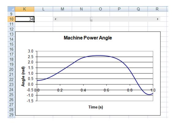
Figure 6: Generator power angle for critical clearance time  $t_{\rm cr} = 0.34$  s. The top portion of the figure displays the scroll bar, which is linked to cell K10.
