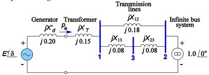
Figure 2: One-line diagram of a synchronous generator connected to a system.
