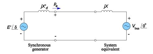
Figure 1: Synchronous generator connected to an infinite bus.
