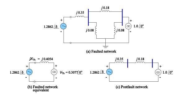
Figure 3: Circuit diagrams for stability analysis: (a) faulted network; (b) Thévenin equivalent of faulted network; and (c) post-fault network, with transmission lines 1–3 and 2–3 removed from the system.
