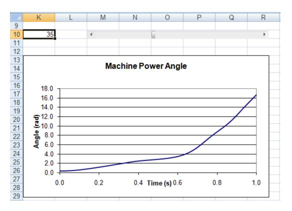
Figure 7: Generator power angle for clearance time  $t_{\rm cl} = 0.35 \text{ s} > t_{\rm cr}$ , where  $t_{\rm cr} = 0.34 \text{ s}$ . The graph clearly shows that this particular clearance time leads to system instability.
