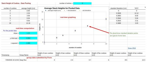
Figure 3: Pooling data in Sheets with real-time graphing and computations including error points (± one standard deviation) for stacking cookies.
